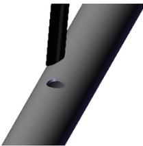
If you are not using a hub dripper, insert the 45° end of the Spaghetti Tube directly into the hole you have created in your lateral hose far enough so the end of the Spaghetti Tube is approximately at the center of the hose. Be careful not to insert it so far that it makes contact with the back wall of the hose. The
