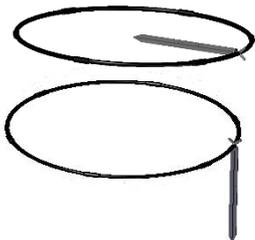
Remove the Pot-Dripper from the box and rotate the stake to a 90° angle from the tubing ring. Be sure you have rotated it in a direction so the hollow 1/8" supply connection points outward from the ring, and the solid 1/8" shutoff barb points into the center of the ring.
